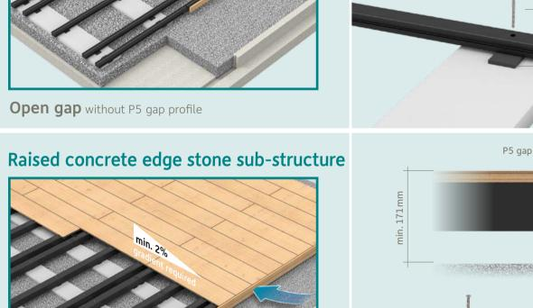
**Closed gap** with groove strip P5 – only with a raised superstructure using a 90 x 90 mm
