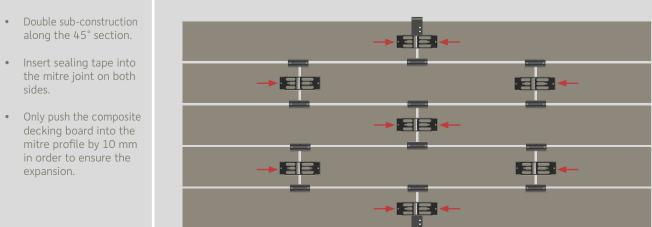
when dealing with heading gaps on the front side. The Distanz Fix is always screwed on to the side of the external composite decking board. The Distanz Fix is not screwed to interior
