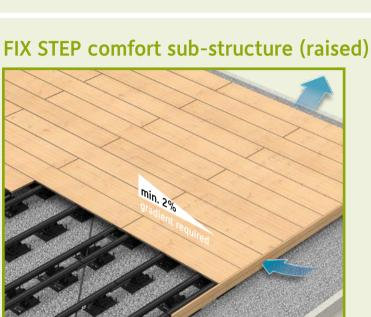
**Closed gap** with groove strip P5\* – Only possible with raised structure at heights of 166 mm and above (third FIX STEP step) provided comfort pad and attachment part are used
